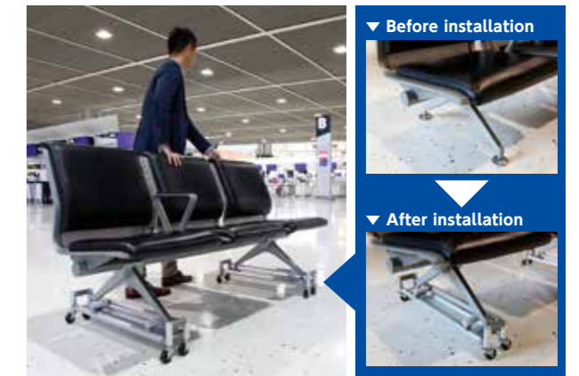
A GF cart for three-seat bench which is used in airport lobbies frequently. Although it is still a prototype, it is easy for one person to carry a bench weighing dozens of kilograms, which reduces loads such as when changing or cleaning seat surfaces, or changing layouts.
