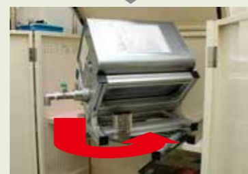
Rotate the frame on the fixed base to the right.
