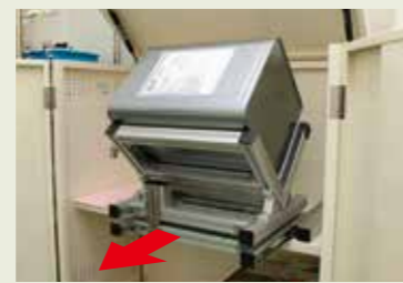
When using it, first pull it forward. Then stop it with a stopper, and fix it at that position.
