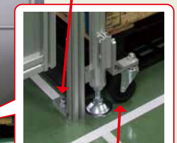
In order to carry in and out material from the back shutter, casters were attached to all the foot suspensions, making it movable.
