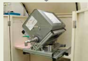
As you rotate 90 degrees, you can pour as it is because the spout is in front. Then just return it with the same process and you are done.
