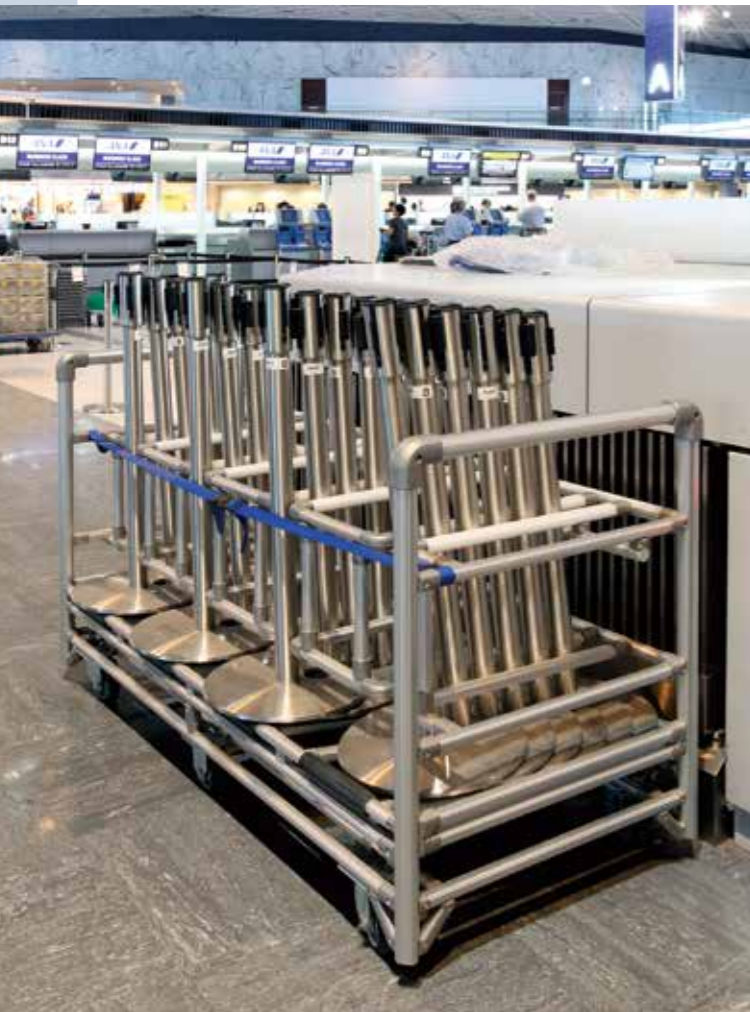
A GF cart that is used in the departure lobby (South Wing) of the Terminal 1. It can hold up to 20 stacking style tape stanchions that can store the base part in layers.
