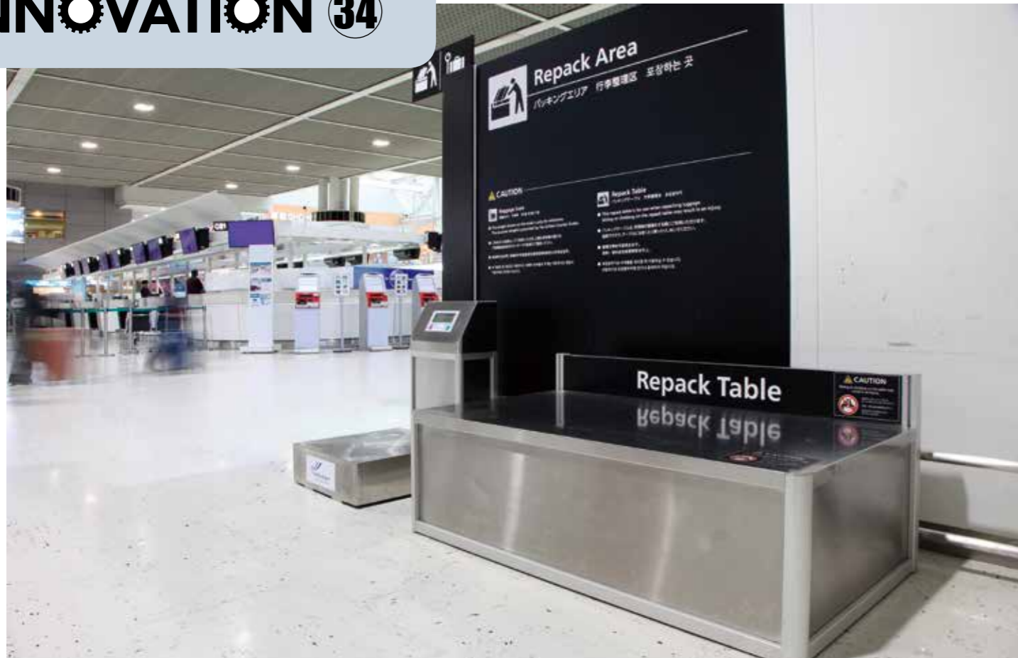
Packing area set in the departure lobby of Terminal 2. The framework of the table was made of SF, and stainless steel was used for the top plate. A weighing scale that fits the design of the table is lined up in the back.
